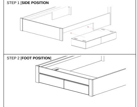
STEP 2 – Carefully slide the Underbed Drawer Unit into its final position under the bed, checking that spacing is even (if installing at the foot) and that drawers are able to open and close smoothly. If using as side storage, we recommend you position your drawer near the foot end to ensure drawers are clear of your bedside table.
