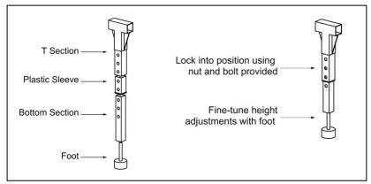
**STEP 3** – Slide the support tube(s) through the spine between slats as per the recommendation on the first page of this guide.
