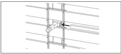
**STEP 4** – Be sure to slide the support tube through the support leg at the same time. Ensure the leg is positioned between the spine as per diagram.
