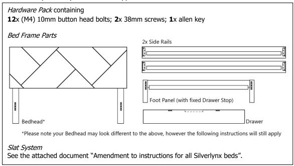
**STEP 1** - Position Bedhead and Side Rails approximately where the bed is to be set up. Connect the Side Rails to the Bedhead by hooking the side rail brackets onto the head brackets.
