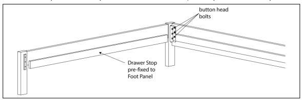
**STEP 4** – Ensure that the bed is sitting square and then tighten all button head bolts using the allen key. Once snug, tighten only with  $\frac{1}{4}$  turn of the Allen Key. DO NOT USE cordless drivers or power drills as over-tightening can cause the foot end rail to bow. After this step your bed should look like the diagram below
