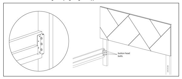
**STEP 3** – Complete the above process on the other side rail, then repeat with the foot panel.
